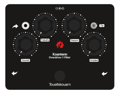
Gounid : Gain Frekañs : Filter Cutoff Frequency Dasson : Filter Resonance Ampled : Volume Tip : High Pass / Low Pass Filter switch Jack 3,5 : Stereo Jack for CV input or expression pedal with a stereo 3,5 to 2 X 6,35 jacks adapter (not provided) Power : 9V/12V DC, negative tip / 25mA
